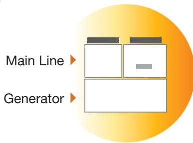
In case of a main line power outage, the ATS\* automatically switches over to the backup line, granting uninterrupted power supply to the unit. The double power supply makes FR-Z suitable for Uptime Institute's TIER III and TIER IV\*\* design topologies, the highest standards of reliability.
